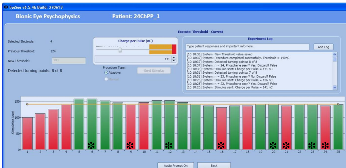
255 256 Figure 4. An example of the up-down staircase procedure used for threshold measurements. 257 Each trial consisted of a pulse train lasting 2 secs. The subject was asked to verbally respond
