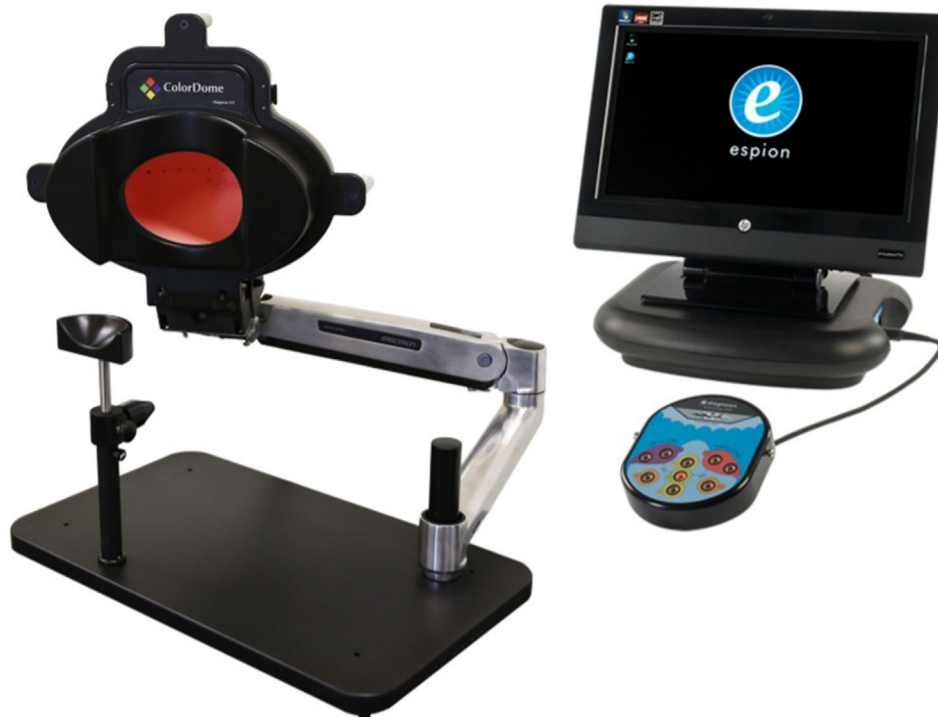
Figure 7. Example of equipment that can be used for full-field electroretinography, the Espion ColorDome LED-based full-field stimulator. 37 New models of the Espion system also include software to enable full-field stimulus threshold testing.
