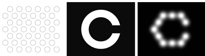
Figure 1. Phosphene rendering for simulated prosthetic vision using the abstract model described by McCarthy et al. 29 Left: electrode layout. Center: input image. Right: phosphene rendering produced by sampling the input image at the electrode locations.
