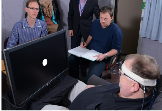
Figure 5: The experimental setting for the light localization task. The participant can be seen with the head-mounted camera directed towards the light localization fixation dot. Participants are free to move their head to scan with the camera. Investigators MP and CM are also visible.
