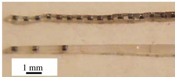
159 160 Fig. 3. Photos of electrode array examples. Top: Nucleus straight array. Bottom: 125 \mu\text{m} optical-fibre- 161 embedded electrode array.
