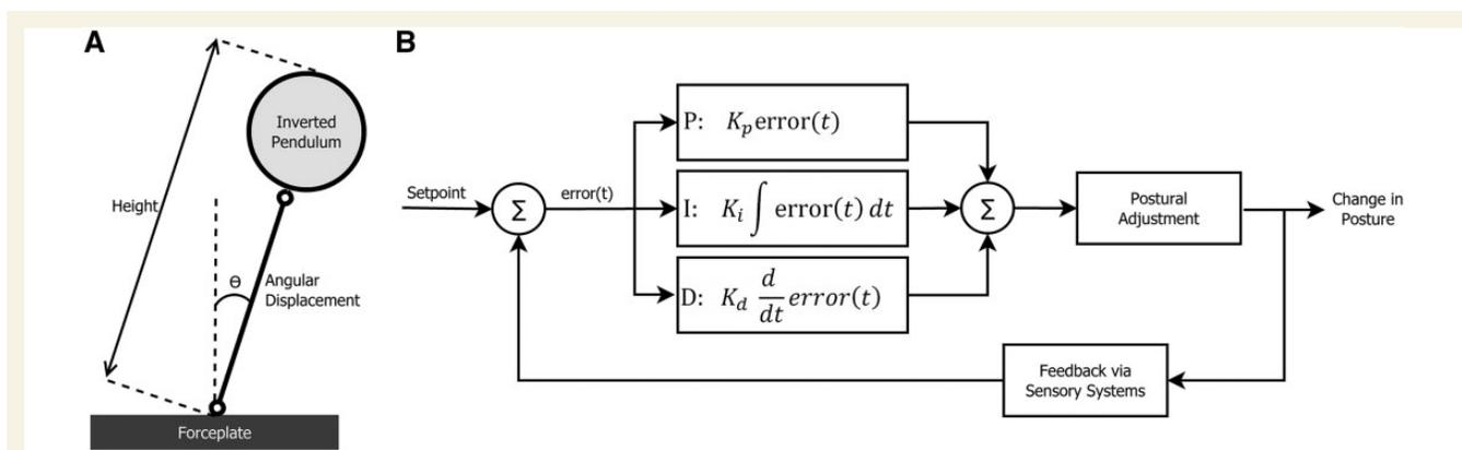
**Figure 2** Schematic showing the inverted pendulum model of human balance (A) used in the PID control system (B). The setpoint input of the PID controller is fixed at zero and acquired posturography time-series data (converted to angular displacement using participant's height) gives the output allowing estimation of the factors  $K_p$  (proportional),  $K_i$  (integral) and  $K_d$  (derivative).
