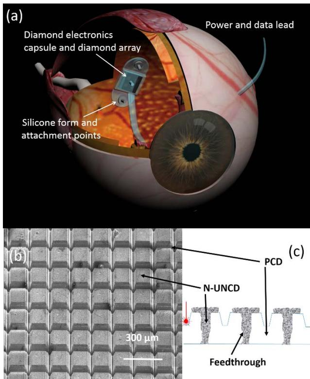
Figure 1. (a) Location and appearance of the BVA retinal prosthesis. (b) SEM image of (b) and internal structure (c) of the PCD / N-UNCD retinal stimulation electrode array.<sup>1, 2</sup>
